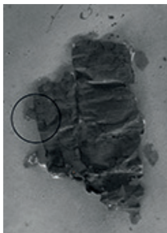
Fig. 3: 3-D image layer of cornice 2 , fragment f5. University of Kentucky, EduceLab. Circled area indicates where the piece broke off and rotated, and clearly shows grain patterns and layers that more clearly indicate the piece's shape.
